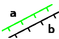
Misgengi a) Mikil vatnafarsleg áhrif b) lítil vatnafarsleg áhrif / Fault a) highly permeable b) slightly permeable
